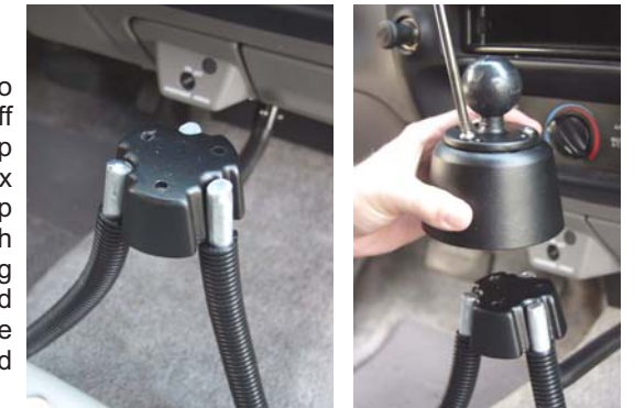
L. 1st Arm attached & bent C. 2nd Arm attached & bent R. 3 Arms attached bent & cut to length
