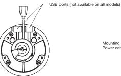
Mounting hole required: 1" (25.4 mm) Power cable length: 39.37" (1.5 m) from exit of stand
