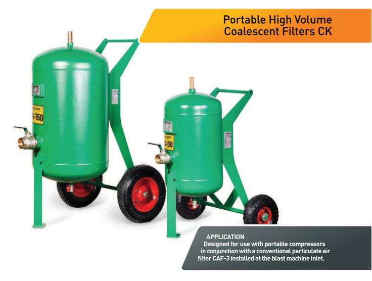
Portable high volume coalescent filters CK-50/150/250 are a most effective solution to remove up to 95% of the liquid condensate and dirt particles, down to 10 microns, from compressed air supply. Specially designed for portable use by sandblasting applications.
