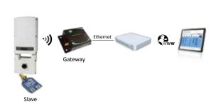
Replacing RS485 inverters interconnections
