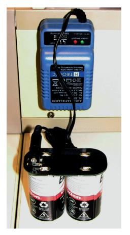
The TRAPMASTER is supplied with a special rechargeable battery. This battery is designed for a very wide temperature range (down to -40°C), in order to ensure reliable trap monitoring even at prolonged minus temperatures.
